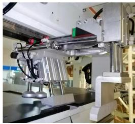
The ELEV8 is LEADING the industry with the ONLY programmable parts back-stop fence allowing for each station to work independent in an in-or-out position. This feature allows the panel to be placed 120mm passed the edge of the table allowing the vertical router 100mm of programmable Y-axis routing. All positions have position sensor monitoring for machine safety.
