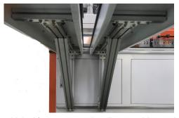
4 **phenolic tables**, 300mm x 1500mm, (12 inch x 60 inch) are mounted on linear guides and can be moved to accommodate large panels or pushed to either side to open up the work space area of the machine. *Making this machine ideal for the closet industry too.*
