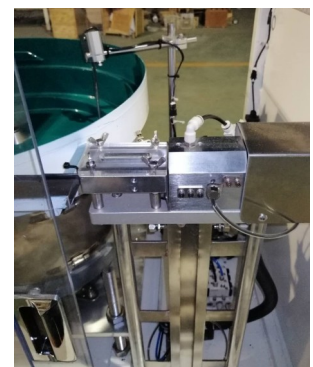
8mm Barbed PD20 connector Vibrator with Auto-Rotating Fastener Feeder.
